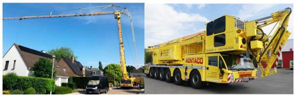
**Example of a foldable tower crane** Specifications: width 2.99M Length 16.5M with crane arm 60M Width crane stable with stamps in Position 7,5M length arm 50M
