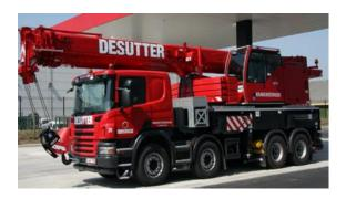
Example of a 60-TON crane Specifications: CRANE 60 TON + extra ballast if needed! width 2.55M Length 9 M and with crane arm 11,5 M Width crane stabled with stamps in Position 7M length arm 9,6 – 43M
