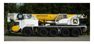
Example of a 100-TON crane Specifications: CRANE 100 TON + extra ballast if needed! width 2.99M Length 12M with crane arm 13,3 M Width crane stable with stamps in Position 7,5M length arm 11,7 – 60M
